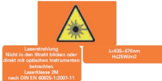
Laser class 2M warning labels on the laser instrument.
